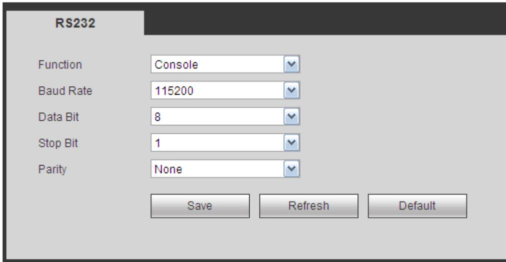
The screenshot shows a configuration window titled "RS232". It features five dropdown menus for configuration: "Function" (set to "Console"), "Baud Rate" (set to "115200"), "Data Bit" (set to "8"), "Stop Bit" (set to "1"), and "Parity" (set to "None"). Below these menus are three buttons: "Save", "Refresh", and "Default".
