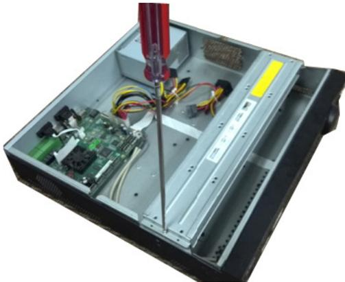
□ Open top cover and then remove the HDD bracket
