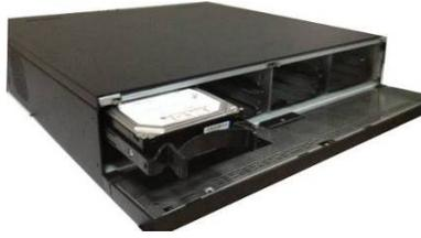
3. Put the HDD to the slot and adjust the handle to secure it.
